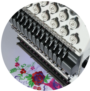
Tension arm guards for added safety
